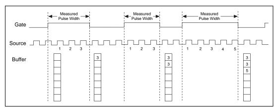
Figure 2-29. Buffered Pulse Width Measurement
